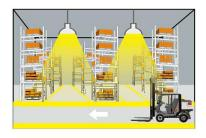
With insufficient ambient light, the sensor switches on the light when motion is detected.
