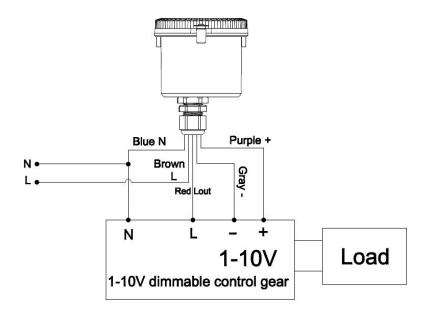
\*The sensor is designed for connect one load only. Connect more than one loads may damage the sensor.
