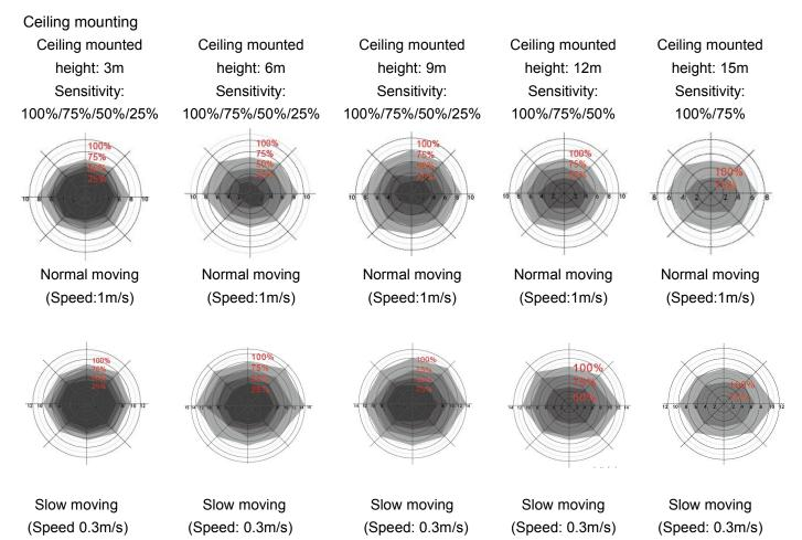
\*Only 100%/75%/50% detection sensitivity is workable when installed at 10m & 15m mounting height. 25% sensitivity is not able to detect motion signal.
