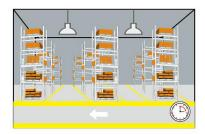
3 After elapse of hold time, the sensor switches off the light when no motion is detected.
