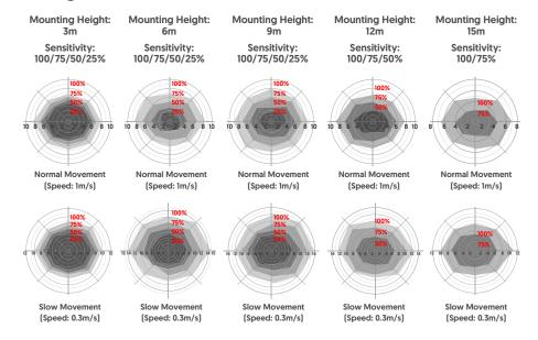
Note: Only 100%/75%/50% detection sensitivity is feasible when installed at 10m or 15m mounting height, as 25% will not detect motion.
