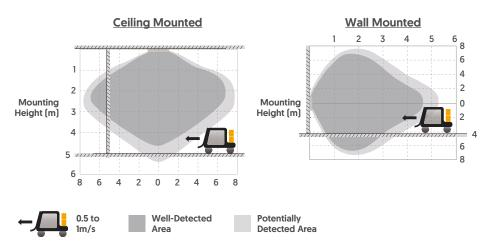
The highest mounting height is ideally 4.5m for optimal detection (see dark grey areas). This figure indicates 100% sensitivity.
