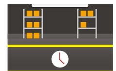
4) After stand-by period elapses, the sensor will switch the light off if no motion is detected.
