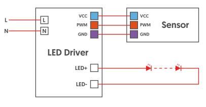
VCC = DC 12V Input PWM = 0/10V DIM+ GND = 0/10V DIM-
