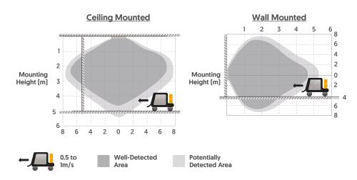
The highest mounting height is ideally 4.5m for optimal detection (see dark grey areas). This figure indicates 100% sensitivity.
