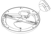
4) Use tools to bend the two installation tabs corresponding with install slots. Make sure the tabs are firmly inside the slots.
