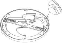
4) Use tools to bend the two installation tabs corresponding with install slots. Make sure the tabs are firmly inside the slots.
