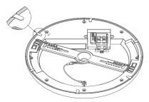
3) Press the installation tabs firmly onto the back surface of the downlight.
