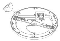
3) Press the installation tabs firmly onto the back surface of the downlight.
